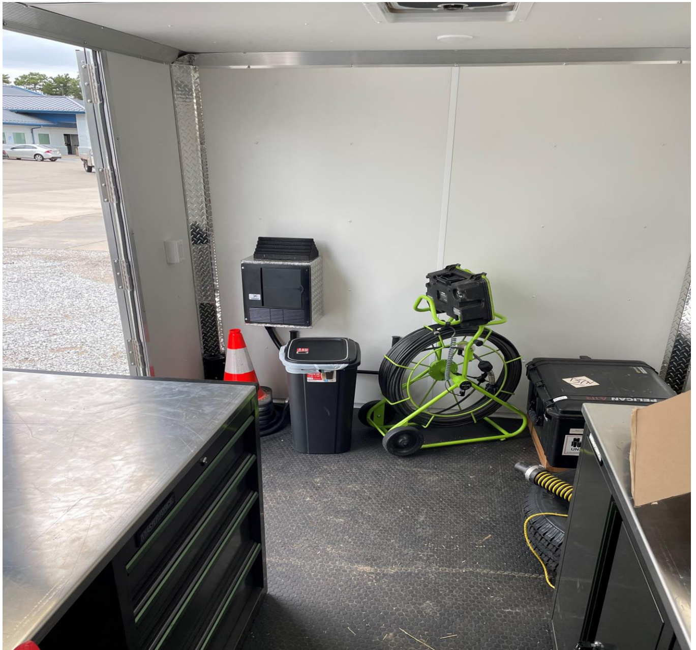
Inside front of trailer showing power box, mobile cabling wheel, underwater camera in a Pelican Box, and tool/accessory cabinets.
