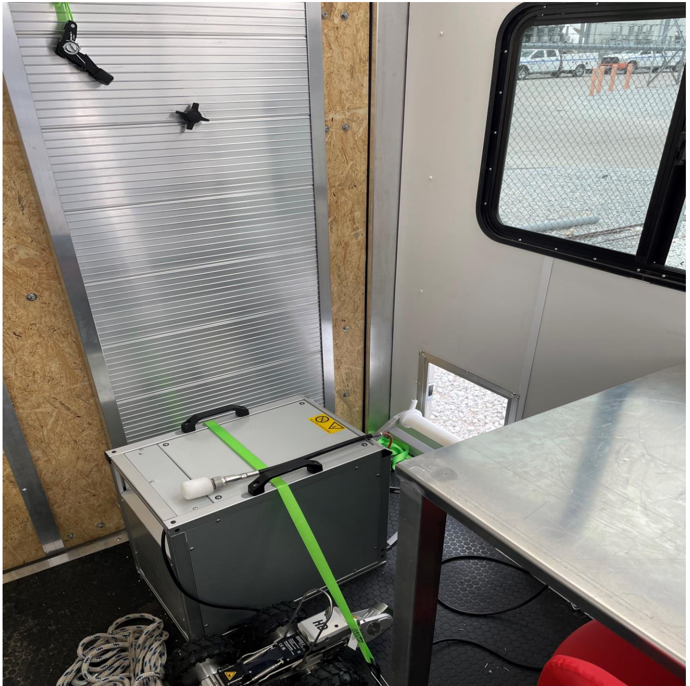
Rear of trailer showing the automated cabling box with small door and crawler camera in the foreground.
