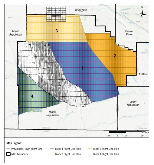
Blocks 3 and 4 were flown during the summer of 2024. This was the final flight for the AEM data collection portion of this grant. All QA/QC data has also been completed for this and is now being processed. Jesse Korus with UNL has been doing data processing to turn this data from resistance values into aquifer properties we can use in a groundwater model. He has finalized all the data processing and has transferred that information to our modeling consultants to
