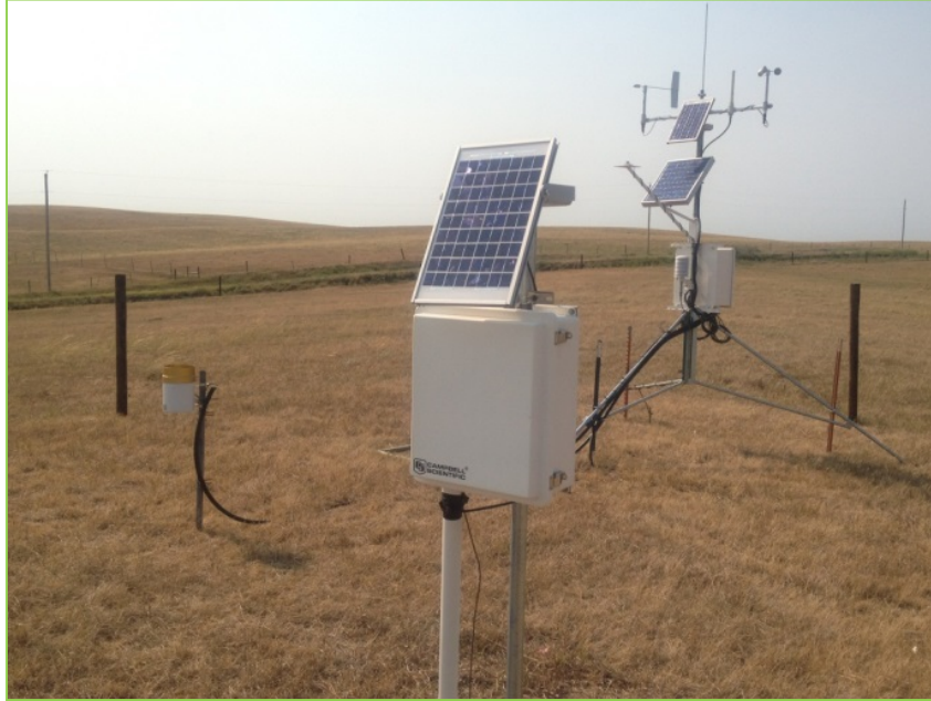
Image 6 Recharge and weather monitoring equipment near Fordyce, Nebraska.
