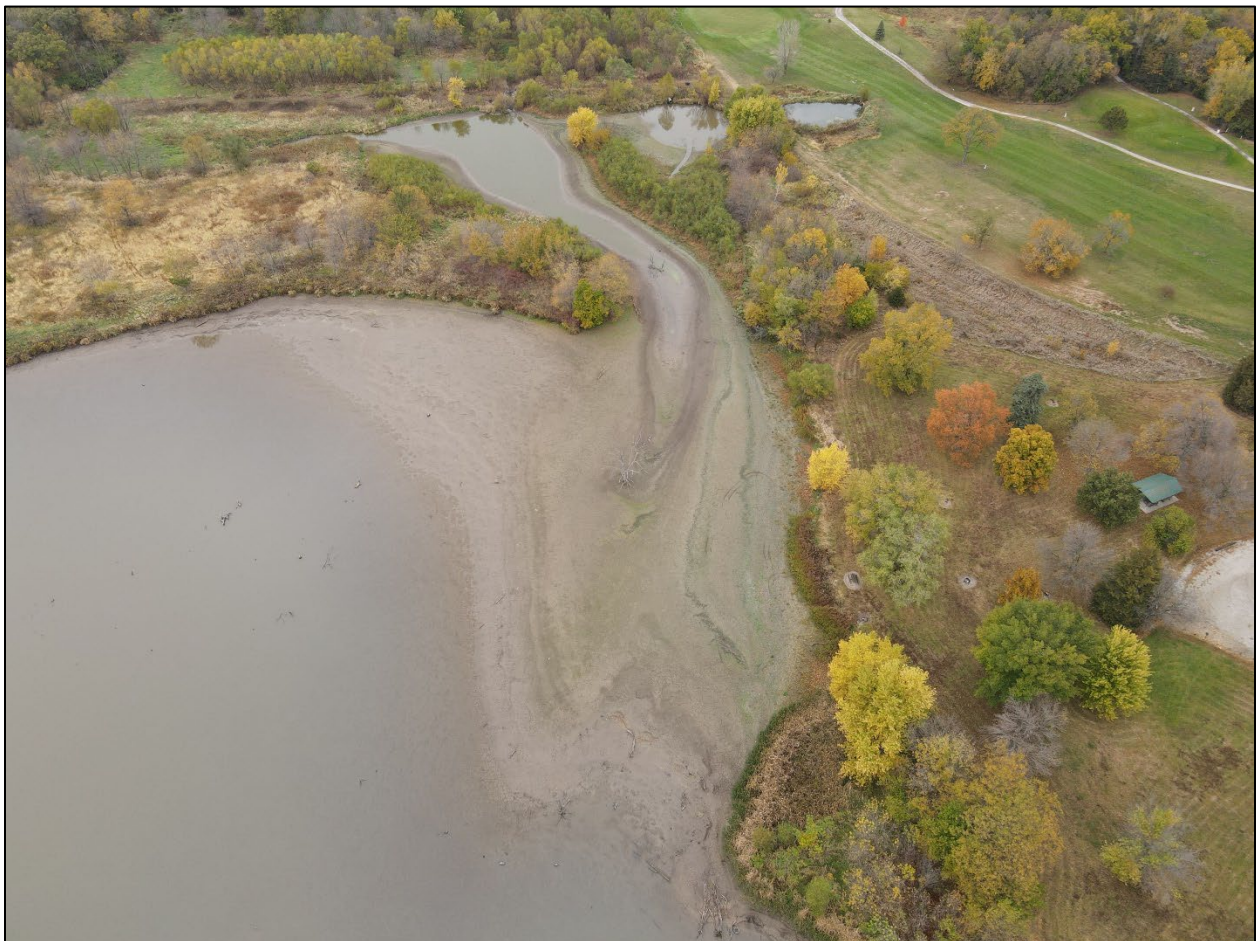
Photo 1. Aerial photograph of sediment accumulated in the headwaters of the lake (2021)
