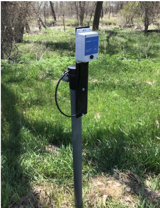
Figure 1 A monitoring well equipped with a pressure transducer and LoRaWAN Paige Wireless device in the TPNRD.
