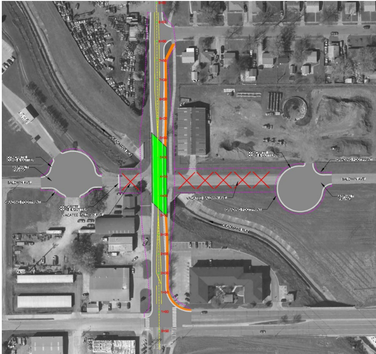
Figure B-1.A.6(4) Baldwin Ave Termination
