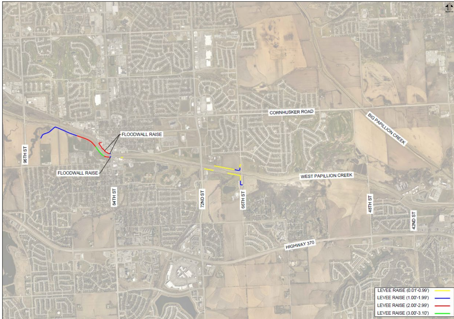
Figure B-1.A.6 - Required Levee Raises with No Modifications to 66th Street Bridge
