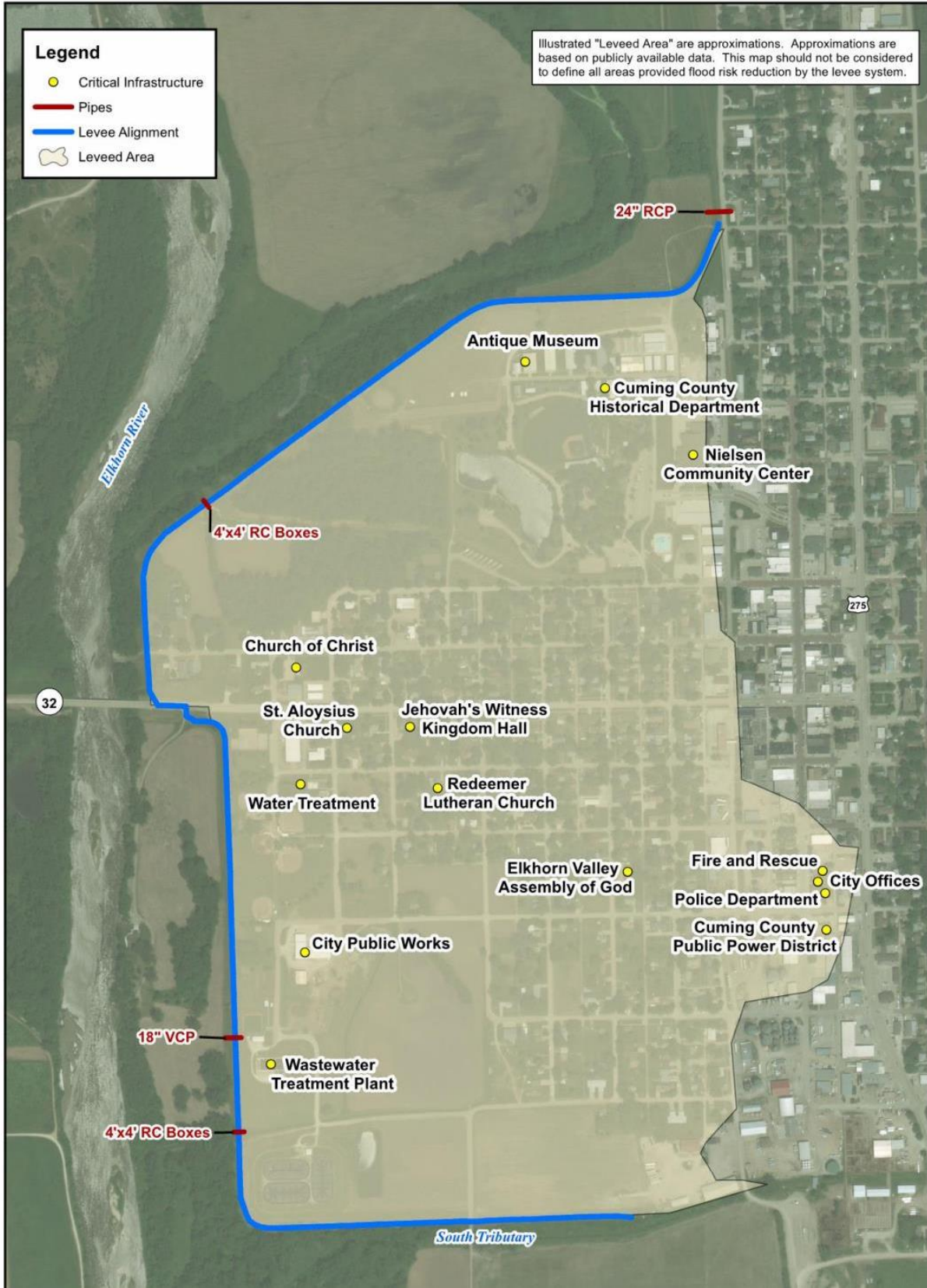
Critical infrastructure at risk within the leveed area.
