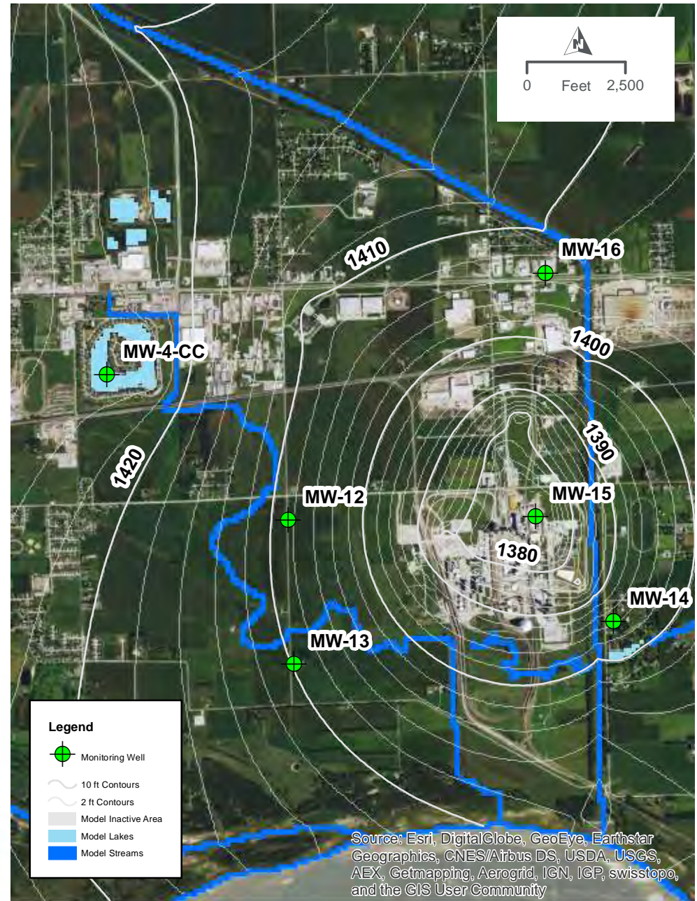
COLUMBUS AREA WATER RESOURCES ASSESSMENT GROUNDWATER HYDROGRAPHS AND MAP WITH CHRISTOPHER'S COVE PROJECT, DEC 2028
