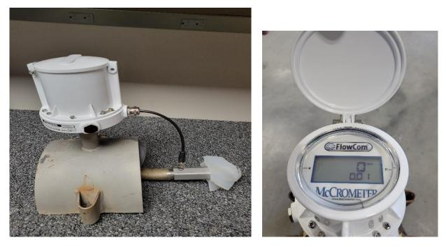
A sensor is installed in the bearing connected to the prop that detects prop revolutions and generates pulses that are translated by the meter head into flow rates based on the programming of the meter. Typically, each prop revolution generates two pulses that are equal to 2.5 gallons. The meter heads are battery operated and have a battery life of an estimated 5-9 years.
