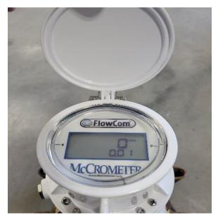
Installing the new meter heads and sensors located within the bearing near the prop of the meters requires removing the meters from the field and bringing them to the shop. This makes it impractical to do any installation during the spring and summer when irrigation is occurring and meters are operating.
